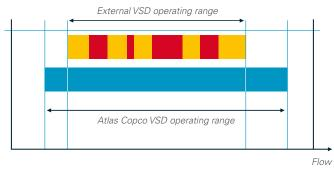
Flow gaps due to vibration and noise issues
