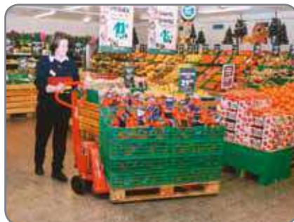
Adjustable fork height - no problems when handling low and worn pallets.
