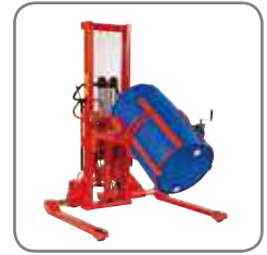
Using a Logiflex without straddle legs, the drum has to be placed on a pallet or other suitable stand above floor level.
