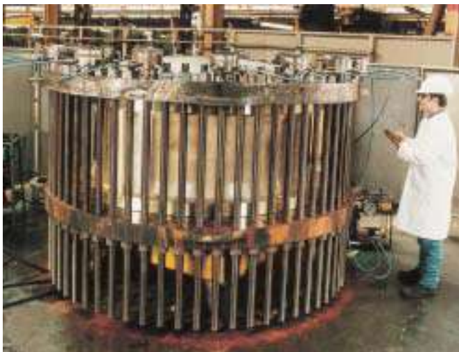
84" 150 lb valve undergoing hydrotest in Goodwin factory
