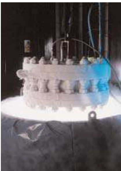
24"ANSI 150lb Check Valve on Cryogenic Test
