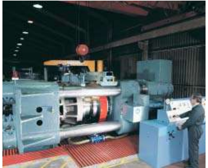
2500 ton hydraulic test rig in Goodwin's Assembly bay
