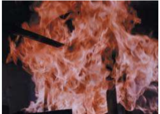
16" 600 lb BFR Flanged Check Valve undergoing firetest
