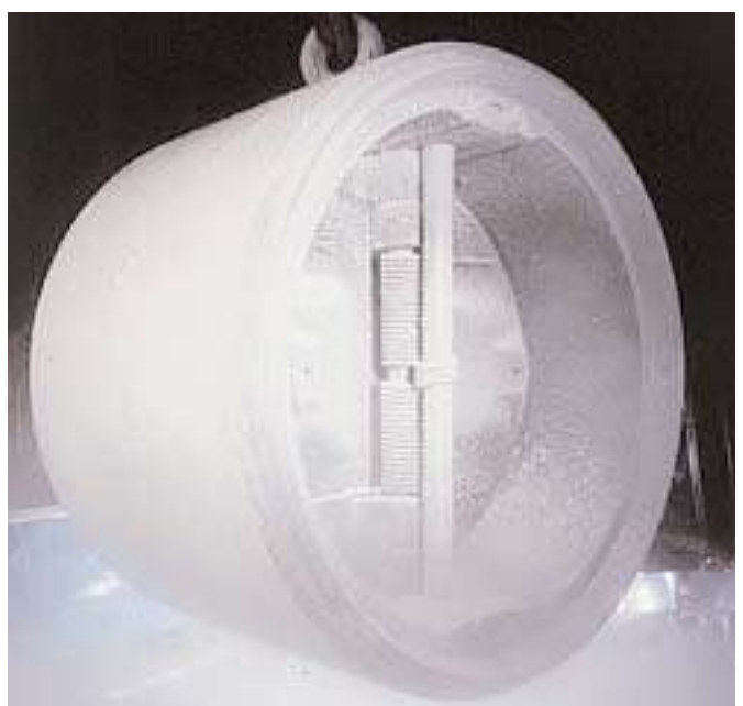
42"ANSI 600# Butt weld end Check Valve after Cryogenic Test with test plates removed.
