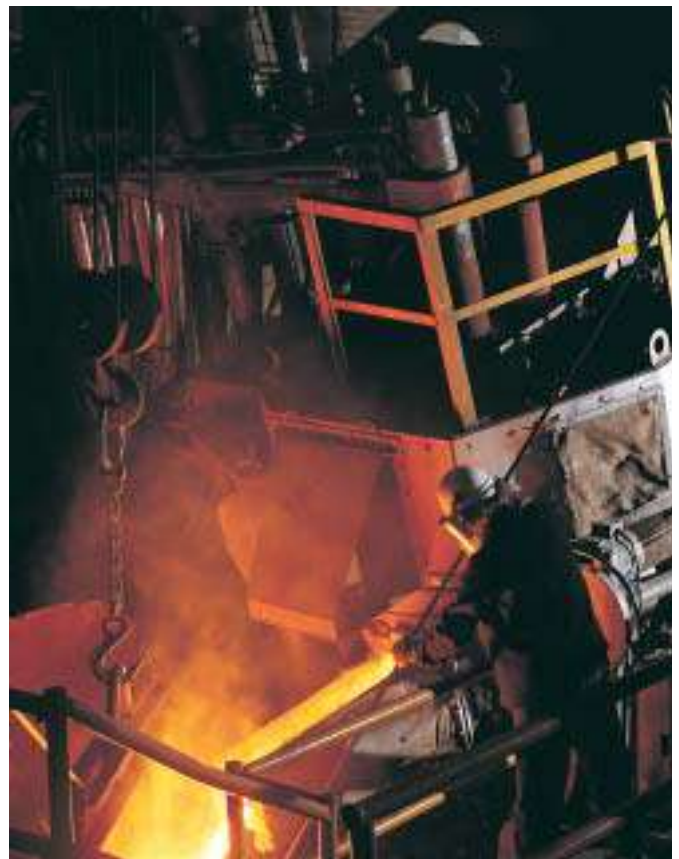
8 ton arc furnace at Goodwin Steel Castings
