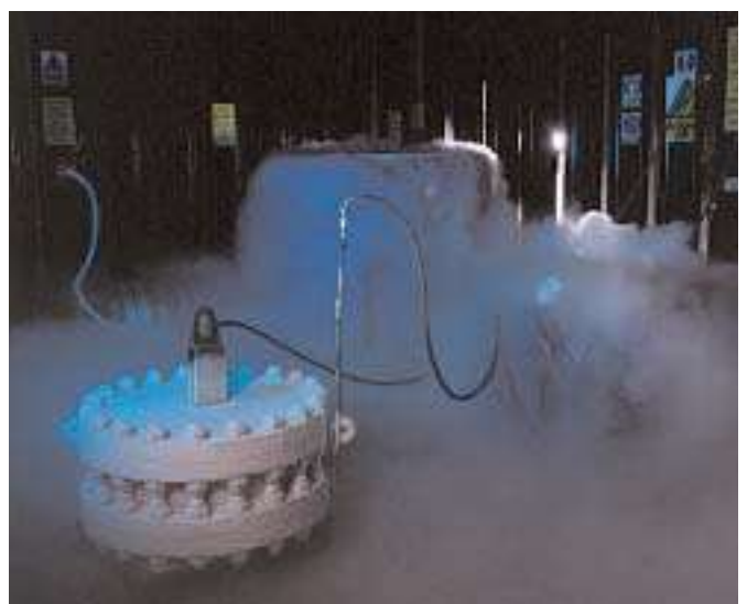
Cryogenic test facility for helium leak testing
