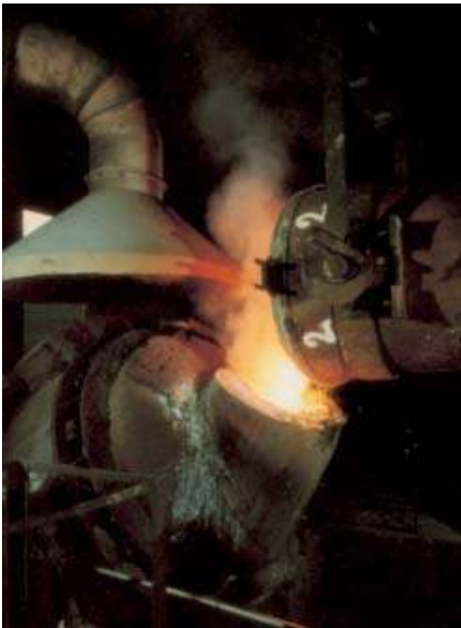
Charging Goodwin Steel Castings 8 ton AOD refining vessel
